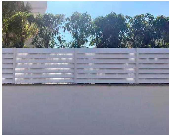
Enclose now your space with a modern, robust and fast construction. It consists of vertical posts and straight lines of cross sections or Z-sections. With a profile that can be placed either with an alternating board or with a board placed on one side. It's strong durable construction guarantees high durability over time, even with no maintenance costs, thanks to the reliability of aluminum.
